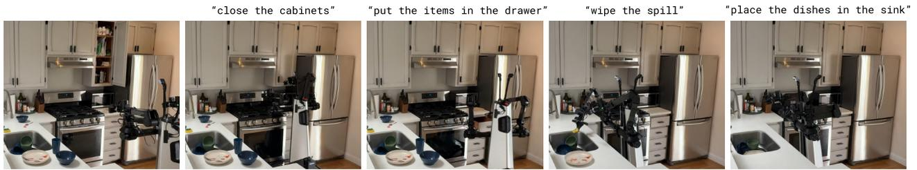
Fig. 2:  $\pi_{0.5}$  **cleaning a new kitchen**. The robot is tasked with cleaning a kitchen in a home that was not in the training data. The model is given general tasks (close the cabinets, put the items in the drawer, wipe the spill, and put the dishes in the sink), which it performs by both predicting subtasks to accomplish (e.g., pick up the plate) and emitting low-level actions.
