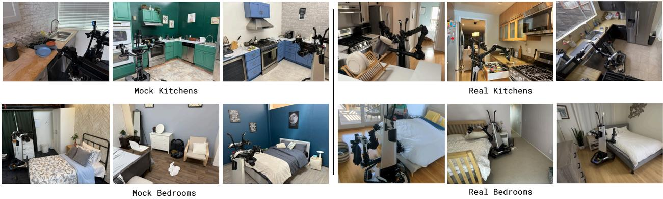
Fig. 6: **Evaluation environments.** We evaluate  $\pi_{0.5}$  in entirely new kitchens and bedrooms that were not seen during training, with novel objects, backgrounds, and layouts. We use a set of mock rooms for controlled, reproducible quantitative comparisons (left) and real homes for a realistic final evaluation (right).
